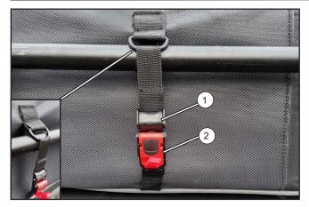
// Insert the lock pin (1) into the lock catch (2).
