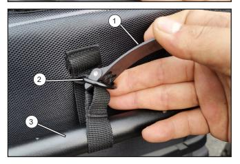
Installation of the soft storage bag requires the rear rack extension (1) to be installed.
