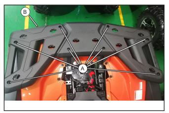
Install the rear rack cover (B) and previously removed screws (A). Hand-tighten the screws sufficiently, using care not to over-tighten.
