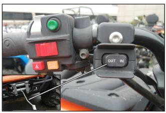
Turn on the main key switch, then press and hold the winch 'OUT' button to let out the winch rope approximately 30cm.
