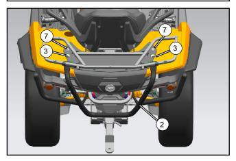
Use a rubber hammer to install the plugs (6) into the rear bumper (2).
