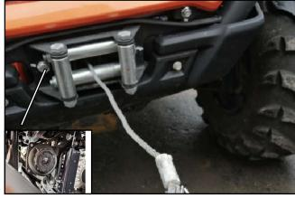
Turn the winch quick release knob to the 'FREESPOOL' position and release the winch cable.
