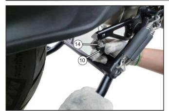
Install the nut (14) on the damping mate assy (10), press the middle supporter assy to a proper position, secure them on the limit seat as shown, then release the middle supporter assy slowly.
