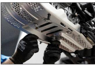
Remove the original skid plate. Discard it and its mounting screws.
