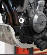
Remove the original plastic panels on the right (A) and left (B) sides. Discard them and their mounting screws.
