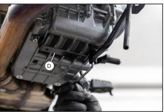
Remove the original lower bracket (D). Discard it and its mounting screws.
