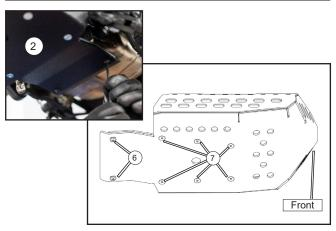
// Install the skid plate (2) using the 8 threaded holes of the inner bracket. Use 6 of the supplied M6x10mm screws (7) and the 2 supplied M6x8mm screws (6), which go in the rearmost holes.
