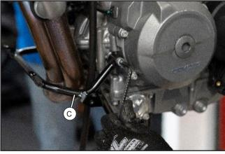
Remove the original front bracket (C). Discard it and its mounting screws.
