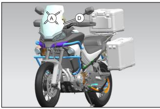
// Install windshield (D) and tighten with screws (A).
