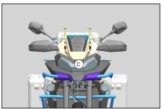
// Remove the screws (C) fixing the windshield bracket.
