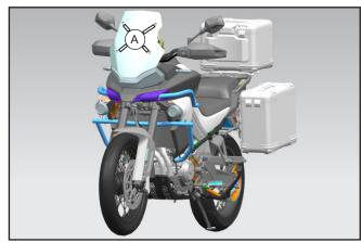
Remove the screws fixing the windshield, remove the windshield (A).
