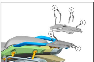
Place the front supports (6) and the rear supports (7) into the assembly position. Install the tray (3) to the rear armrest cover with bolts (4,5). Torque the bolts evenly to specification.
