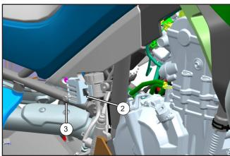
Place the rear fluid reservoir guard (2) into the assembly position and install the bolt (3).
