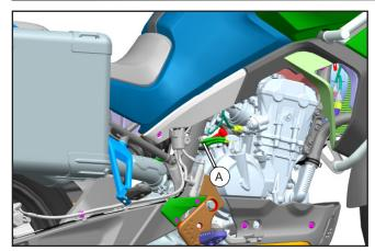
Remove the rear fluid reservoir bolt (A).
