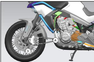
// Place the front brake caliper left guard (3) into the assembly position, install the screws (A) and tighten.
