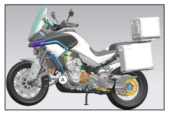
Remove the screws (A) securing the left and right callipers.
