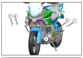
Remove the plugs (C) and bolts (B) in turn, and then remove the front bumper support rod (A).
