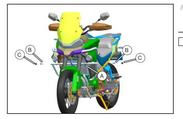
Install the front bumper support rod (A) back to its original position, fasten it with bolts (B), and then plug in the plugs (C).
