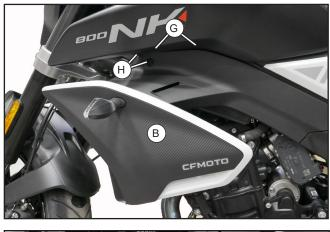
Reinstall expansion rivets (G) and screws (H) for the left side deco plate (B).
