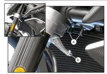
Locate the mounts (A) on the frame and the mount (B) on the lower triple clamp for the steering stabilizer.
