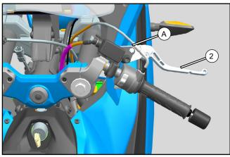
Put the brake lever (2) into the original lever and tighten with bolt (A).
