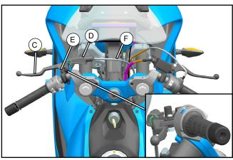
Move the rubber dust cover (D) backward and remove the screw (E) and clutch cable (F) in turn. And finally remove the lever (C).
