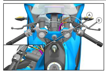
Remove the bolt (A) and lever (B).
