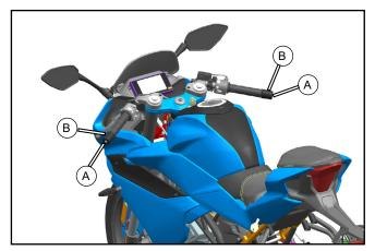
Remove the screws (A) and the balance blocks (B) in turn.
