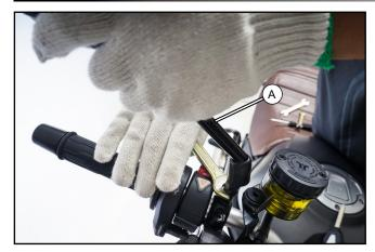
Remove the original left and right rear-view mirrors (A).
