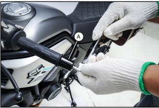
Remove the original left and right balancers (A).
