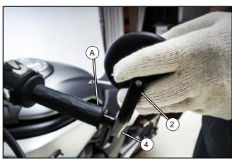
// Install the left and right rear-view mirrors (2,3) to the handlebar with screws (4) and tighten.
