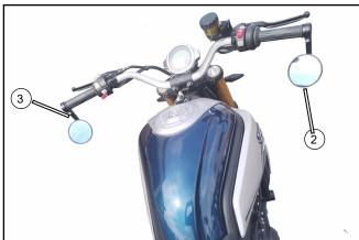
The angle of the rear-view mirror (1) can be adjusted according to the rider's posture.
