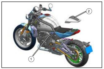
Insert the key (1) into the seat lock and open it, and remove the rear plastic cover (2).
