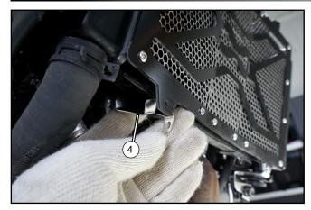
Place the right lower bracket (4) in the assembly position.
