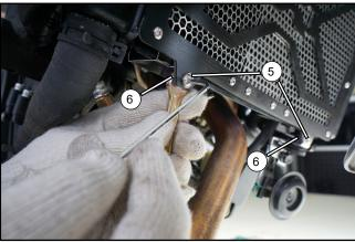
Install screws (5) and nuts (6) and tighten.
