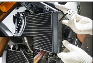
Lift up the radiator (A), and then pull it in the opposite direction of the upper mounting point to reserve the installation position.
