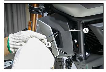
// Loosen the screws (B) and remove the radiator protector (A).
