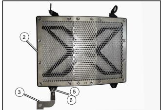
// Install the lower left bracket (3) to the radiator guard (2) with screws (5) and nuts (6). Do not tighten them at this time.
