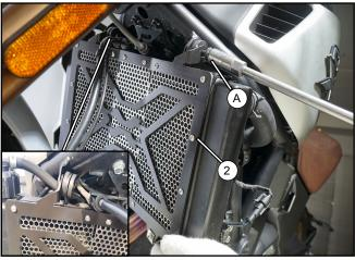
// Install the radiator guard (2) to the radiator with bolt (A).
