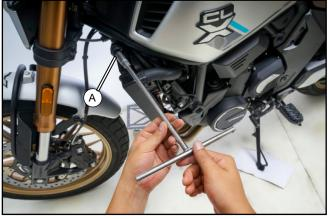
Remove the radiator mounting bolt (A).
