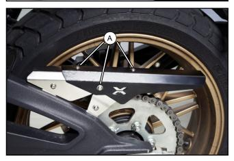
The length of the chain guard can be adjusted by adjusting the screws (A).
