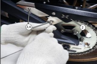
Install the chain panel (2) with washers (3) and screws
