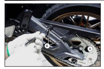
Loosen the bolts (B) and remove the chain guard (A).
