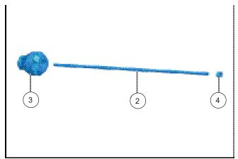
Install a M6 nut (4) on the shorter-thread side of the front axle slider shaft (2). Then insert this shaft through a hinch ball (3) until the ball and nut are on the same side.
