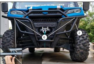
// Install the plugs B (6) into the front bumper (2).
