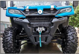
Remove the front bumper panel bolts (A). NOTE: Bolts will not be reused. Discard properly.
