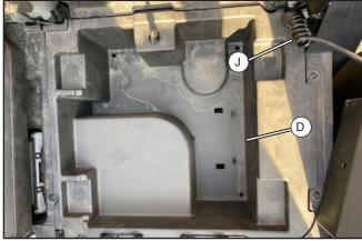
Position the heated driver seat cable (J) as shown in the image and install the seat left lower guard (D).
