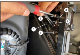
Place the seat heating switch (4) into the opening made under the seat, then secure it with the heating switch bracket (3) and self-tapping screws (5).
