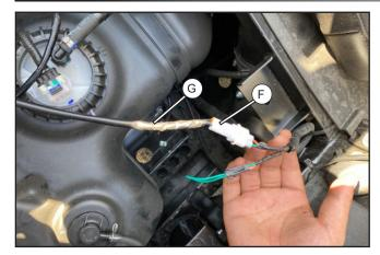
Connect port (F) to port (G) of the seat heating switch.
