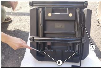
Place the driver seat assy (A) on a protected stable work surface and remove the bolts (B) shown.
