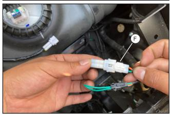
In the vehicle, locate and remove the white plug from reserved port (F) as shown.
