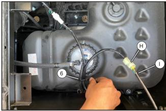
// Connect the seat switch port (H) to the seat heating port (I), and secure them with tie band (6) as shown.
