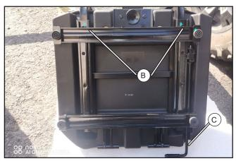
Turn the handle (C) to adjust the seat base position, creating access for removal of the remaining upper bolts (B).
