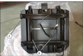
Position the heated driver seat (2) in the assembly position. Install the removed bolts (B) to secure it, using caution not to over-tighten them.
