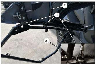
Attach the right door bracket (3) to the right door frame (F) using bolts (6). Torque the fasteners to specification.
