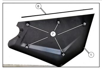
Install nut clips (7) and sealing strip (8) to the left lower door insert (1).
