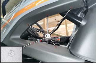
Drill holes in the rear left side door panel opening according to the molded hole trace marks (G) as shown.
