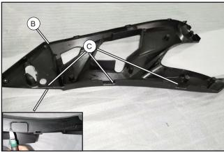
Trim rectangle pieces (C) from the inner door panel (B) as shown, following the lines molded into the panel.
