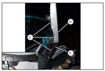
Trim rectangle pieces (C) from the outer door deco panel (D) and outer door rear panel (E) as shown, following the lines molded into the panel.
