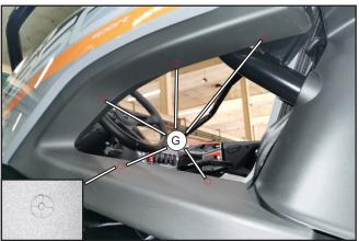
Drill holes in the rear right side door panel opening according to the molded hole trace marks (G) as shown.
