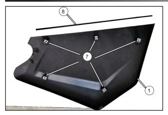
Install nut clips (7) and sealing strip (8) to the right lower door insert (1).
