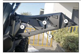
// Remove bolts (A) and driver side inner door panel (B).
