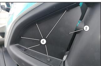
// Install the left door insert panel (2) in the left side door rear panel opening and secure it with plastic clips (4).
