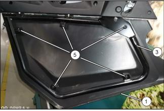
Fasten the right lower door insert (1) to the bracket (3) using inner hex screws (5). Torque the fasteners to specification.
