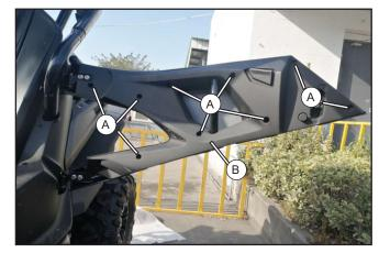
Remove bolts (A) and passenger side inner door panel (B).
