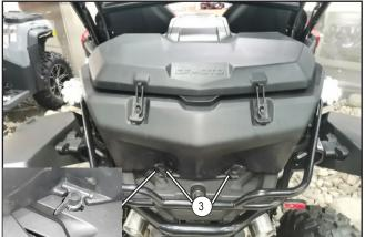
Position the rear cargo box (2) on the rear rack cover (A).
