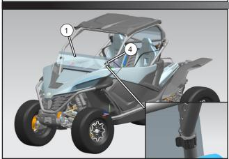
Position the half windshield assembly (1) on the top bar front assembly as shown to determine the clamp positions, then assemble each side with clamps 42 (4). Tighten the screws sufficiently, using care not to overtighten.
