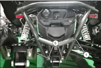
Position the bumper assembly (1) on the rear of the vehicle as shown, then insert inner hex screws (5) but do not tighten at this time.
