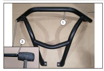
Use a rubber hammer to install the plugs (3) into the rear bumper (1).
