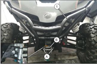
Position the bumper assembly (1) behind the cable pulley (B) as shown. Reinstall the cable pulley bolts (A) but do not tighten them at this time.
