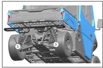
// Install bolts (3) and torque the bolts evenly to specification.
