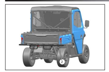
Position the rear bumper (2) in the assembly position as shown.
