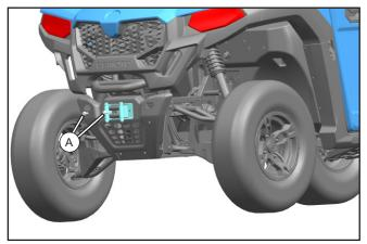
// Remove the winch fairlead bolts (A).
