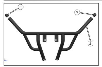
// Use a rubber hammer to install the plugs (3) into the front bumper (2).
